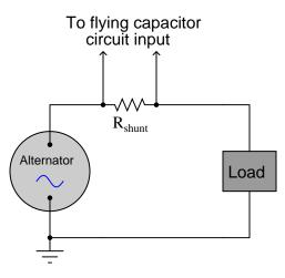
The frequency of the alternator's output is 50 Hz. How does this affect the design of the flying capacitor circuit, so we ensure a fairly accurate reproduction of the AC signal at the output of the flying capacitor circuit? Generalize your answer to cover all conditions where the input signal varies over time.
