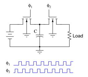
Note: the  $\phi_1$  and  $\phi_2$  pulse signals are collectively referred to as a non-overlapping, two-phase clock.
