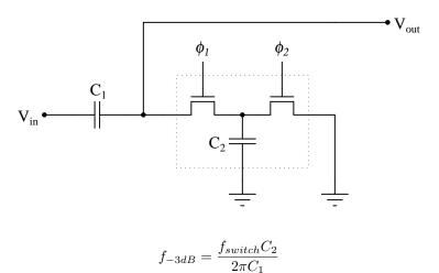
Note: in order for this circuit to be practical,  $f_{switch} >> f_{signal}$ .
