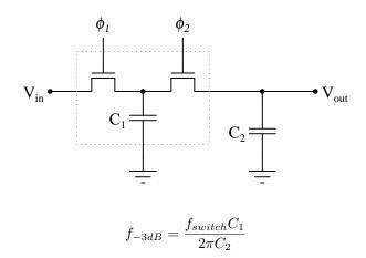
Note: in order for this circuit to be practical,  $f_{switch} >> f_{signal}$ .
