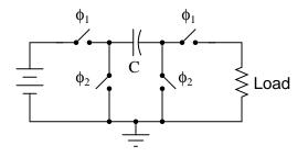
Identify the polarity of voltage across the load resistor in the following switched capacitor circuit. Note: the only difference between this circuit and the last is the switching sequence.
