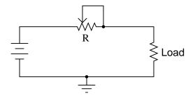
It should be obvious in this circuit that the load current decreases as variable resistance R increases. What might not be so obvious is that the aforementioned switched capacitor circuit *emulates* the variable resistor R in the second circuit, so that there is a mathematical equivalence between f and C in the first circuit, and R in the second circuit, so far as average current is concerned. To put this in simpler terms, the switched capacitor network behaves sort of like a variable resistor.
