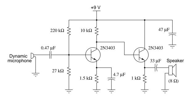
Identify the role of the following components in this audio amplifier circuit:
