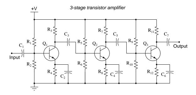
Explain how you would use the "divide and conquer" or "divide by two" strategy of troubleshooting to locate the amplification stage where the fault is. (This is where you divide the signal path into different sections, then test for good signal at points along that path so as to narrow the problem down to one-half of the circuit, then to one-quarter of the circuit, etc.)
