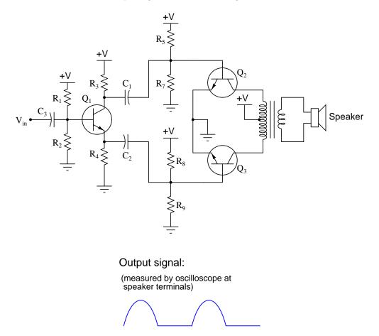
List some of the possible faults in this system, based on the output signal shown by the oscilloscope. Also, determine which components, if any, are known to be good based on the same data:
