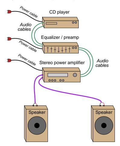
The CD player generates the audio signal to be amplified, while the equalizer/preamp modifies the tone of the signal to suit the listener's preferences and the power amplifier provides adequate power to drive the speakers.
