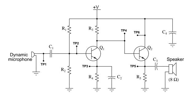
Then, determine whether the DC voltage at each test point  $(V_{TP1} \text{ through } V_{TP6})$  with respect to ground will increase, decrease, or remain the same for each of the given fault conditions:
