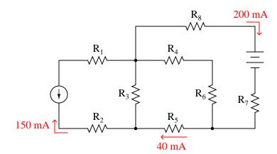
Note: all current arrows point in the direction of electron flow!
