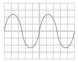
Vertical sensitivity = 2 volts/div 1:1 probe DC coupling Timebase = 0.5 ms/div
