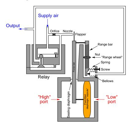
What would have to be done to it to re-calibrate it for a new range of 100 to 350 inches water column?
