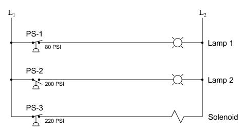
Determine the statuses of these loads at a pressure pressure of 210 PSI.
