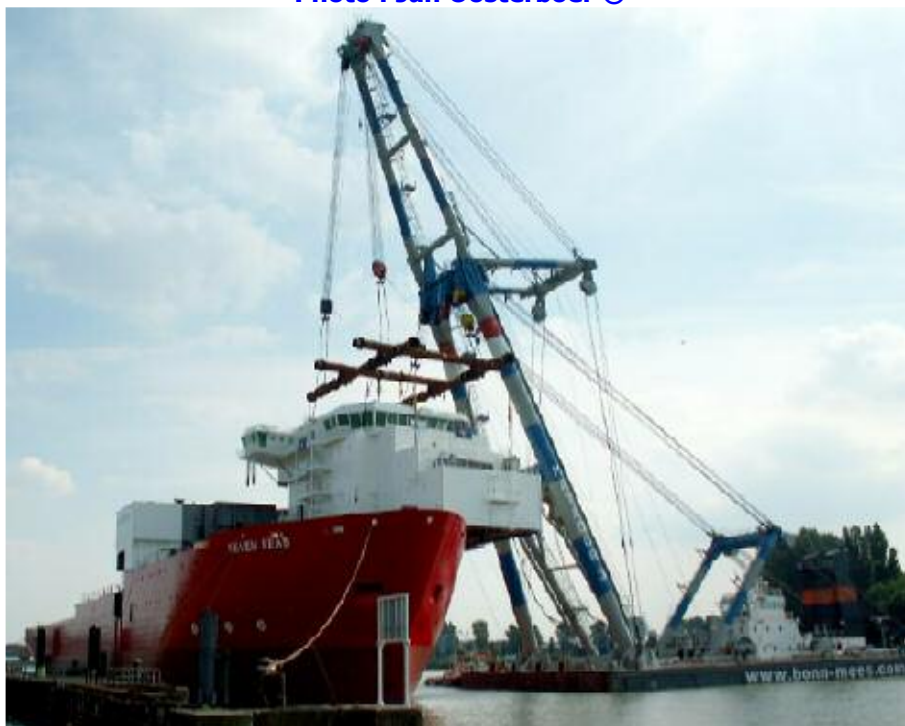
At the Heysehaven the superstructure was lifted onboard the SEVEN SEAS by the sheerlegs MATADOR 3 Photo : Jan Oosterboer ©
